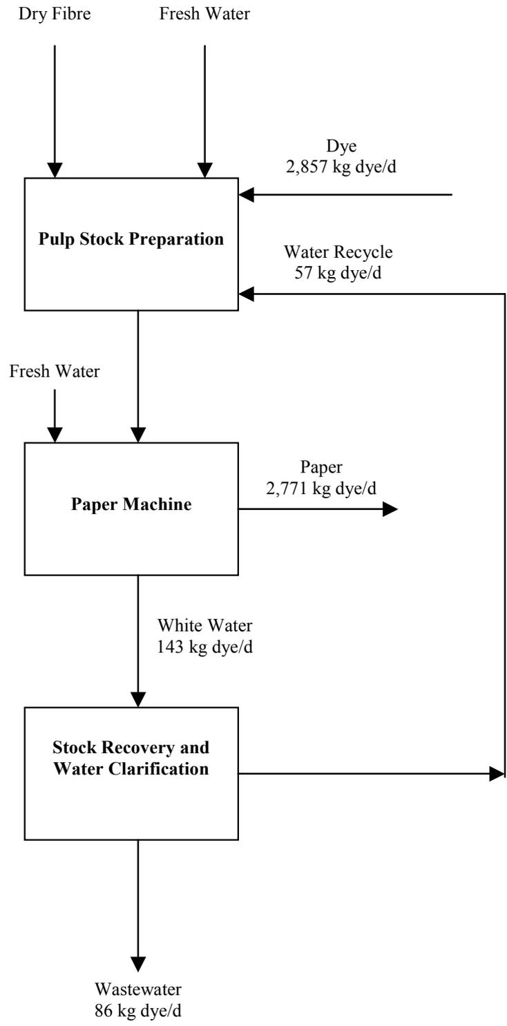
**Figure A.6 – Mass Balance on Dye Determined for Paper Mill by ESD Method**
