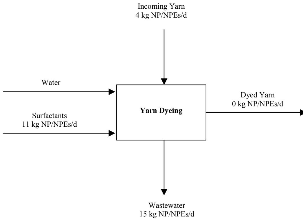
**Figure A.3 – Mass Balance on NP/NPEs Determined for Yarn Dyeing by PRTR Method**
