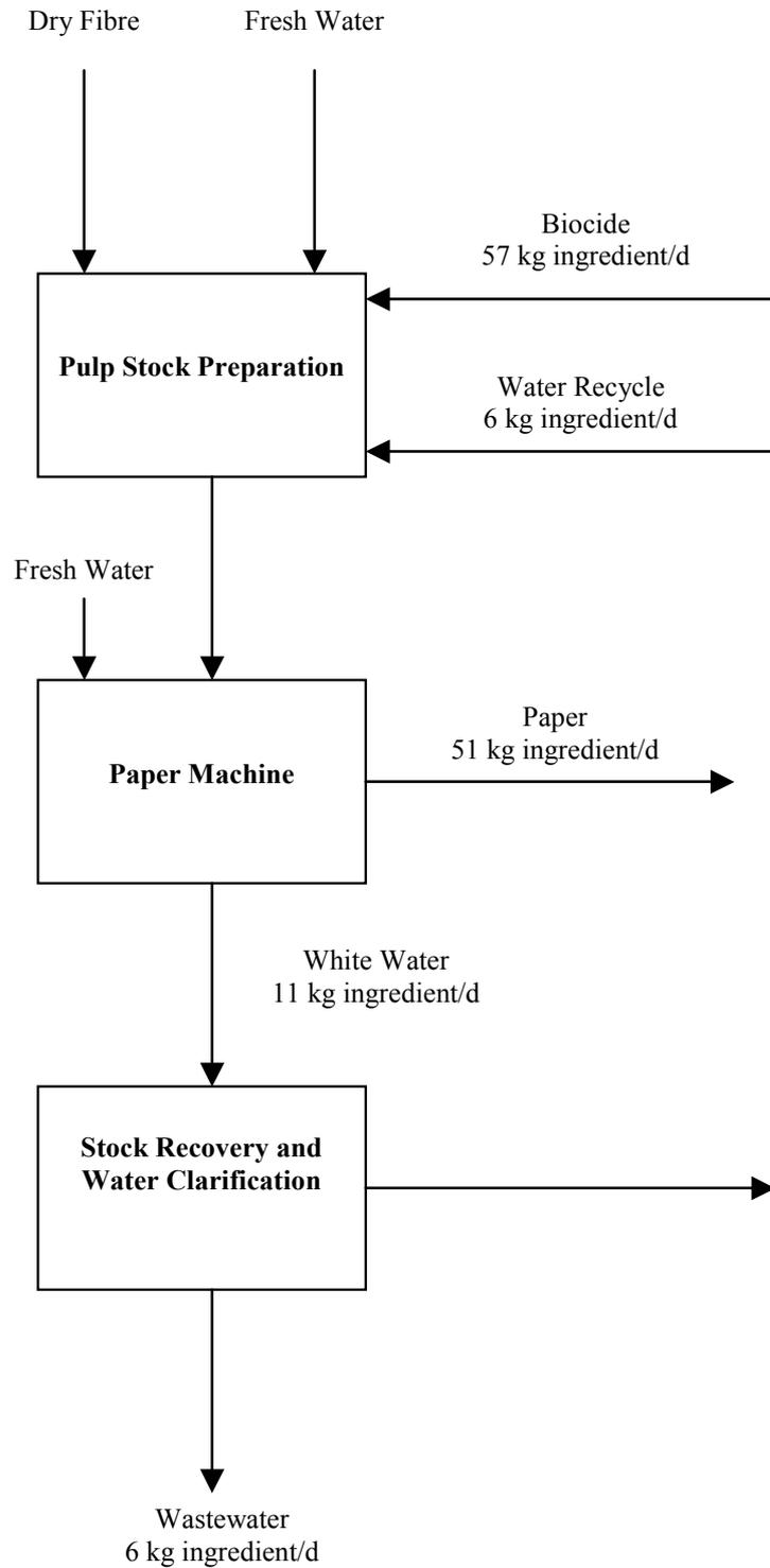
**Figure A.2 – Mass Balance on Biocide Determined for Paper Mill by ESD Method**
