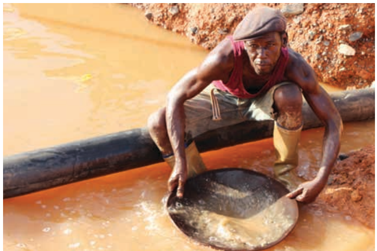
ARTISANAL MINERS USE MERCURY TO SEPARATE GOLD FROM SEDIMENT IN OMAI, ESSEQUIBO, GUYANA. PHOTO BY CHIKA OHASHI, UNDP GUYANA.
