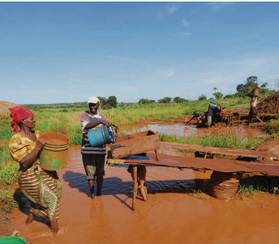
MINERS SEPARATING GOLD FROM SEDIMENTS IN ASGM OPERATIONS IN SHINYANGA, TANZANIA. PHOTO BY AFRICA924/SHUTTERSTOCK.COM.
