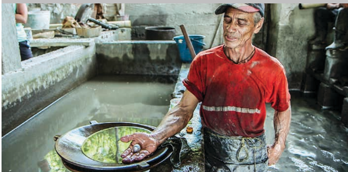
MINER DEMONSTRATING THE USE OF MERCURY IN ASGM IN SEGOVIA, COLOMBIA. PHOTO BY PATRICK FRIES.
