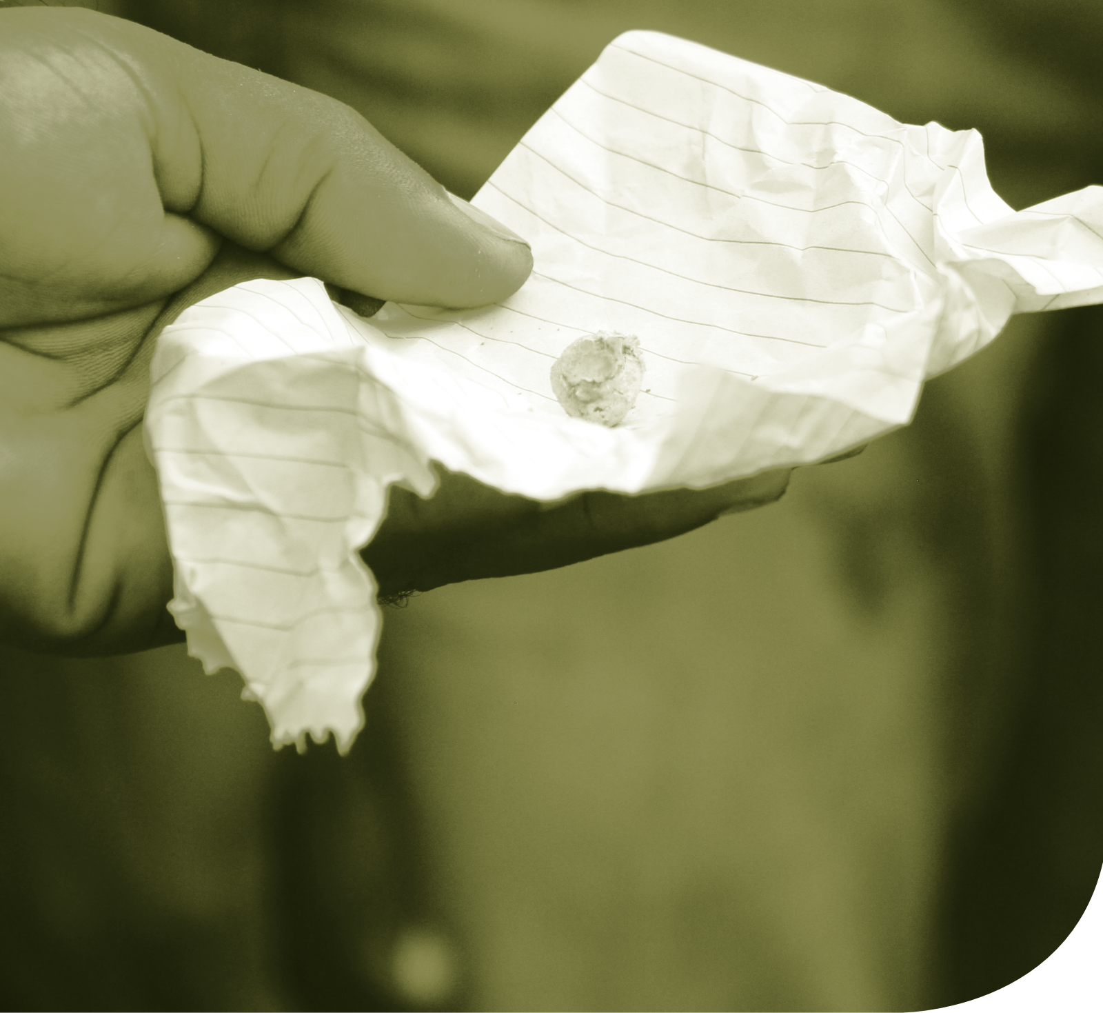
Sponge gold: the output of the burning step in ASGM when amalgam is heated to separate mercury from the gold.
