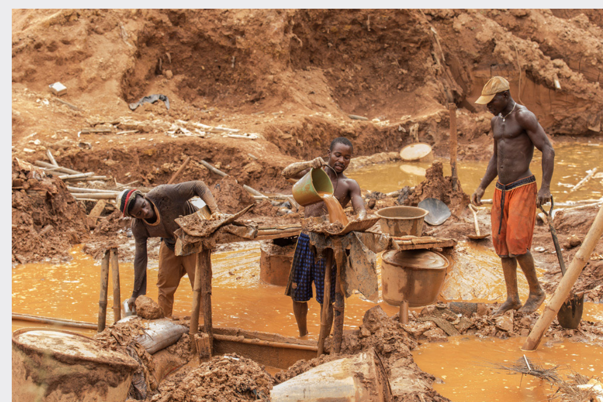
artisanal small-scale gold mining (amalgam process)
