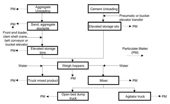
**Figure 1. Basic Process Steps for Concrete Batching** (Source:USEPA *AP-42*, 1995)
